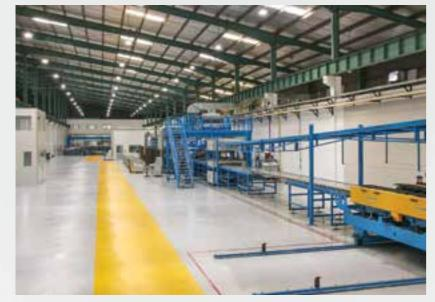
The Panel (PIR) production line, sourced from ITALY, with modern technology is currently operational at the Panel Manufacturing Plant - Greenpan Joint Stock Company.
